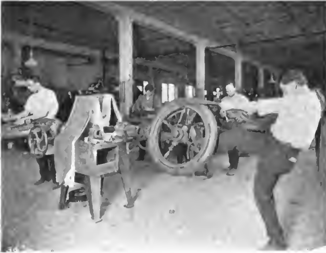
Old Way of Stretching the Fabric on the Core by Hand
